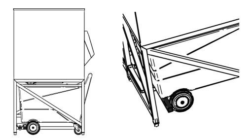
Immediately after, lock the wheels of the cart. To do this, lower the levers on the rear wheels of the cart. Use your foot to press the levers down.
