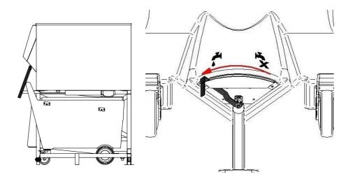
Once all the water has drained out of the cart, close off the valve.
