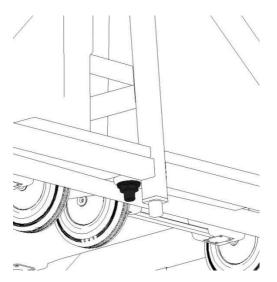
Place the bent end onto the connection at the bottom of the ice storage bin by force-fitting. The other part will go to an outside drain.
