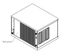
3) Clean the condenser using a vacuum cleaner, soft brush, or low-pressure air. Clean from bottom to top, not side to side. Be careful not to bend the fins of the condenser
