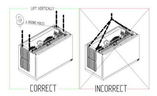
For the lifting and transport of the rest of the models, suitable equipment or machinery must be used for this purpose, such as pallet trucks, forklifts, etc., to ensure the lifting of the machine without causing any damage to the equipment or personnel carrying out the operation. The equipment must be properly packed and protected to avoid cosmetic or mechanical damage during transport.
