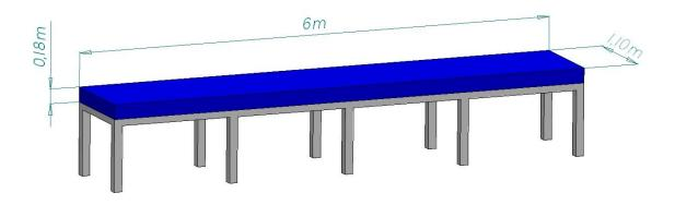
The volume of ice required is 6 m x 1.1 m x 0.18 m = 1.19 m3 of ice
