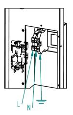
Terminal connector to supply electrical power to the remote condenser, located behind the metallic cover.
